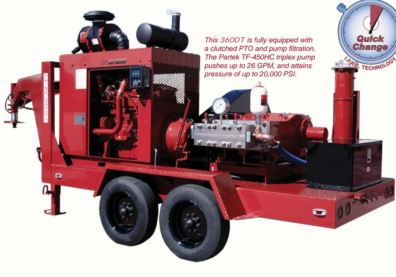
*This 360DT is fully equipped with a clutched PTO and pump filtration. The Partek TF-450HC triplex pump pushes up to 26 GPM, and attains pressure of up to 20,000 PSI.*
