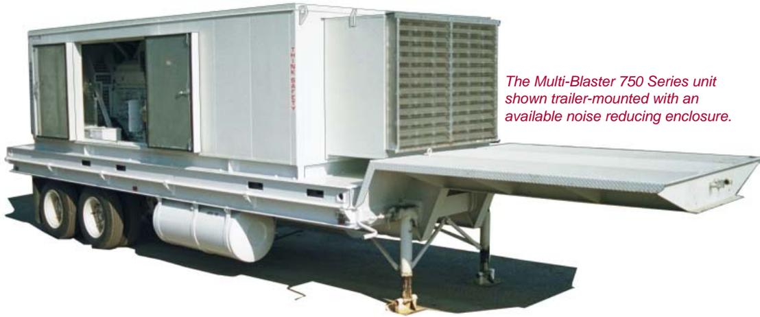
The Multi-Blaster 750 Series unit shown trailer-mounted with an available noise reducing enclosure.
