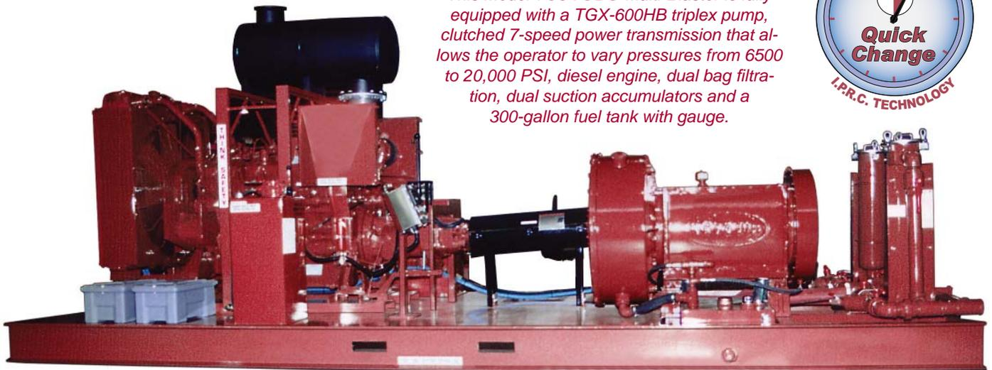
*This Model 760VSDS Multi-Blaster is fully equipped with a TGX-600HB triplex pump, clutched 7-speed power transmission that allows the operator to vary pressures from 6500 to 20,000 PSI, diesel engine, dual bag filtration, dual suction accumulators and a 300-gallon fuel tank with gauge.*
