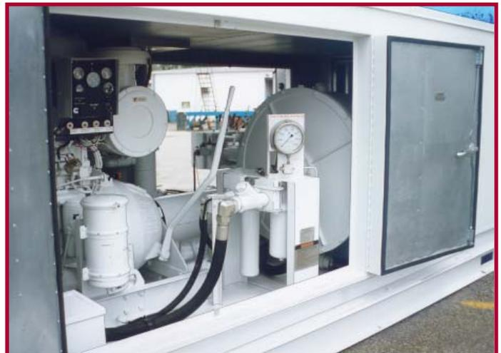
*The Multi-Blaster 750 Series whisperizing cabinet allows access for ease of service from any angle.*
